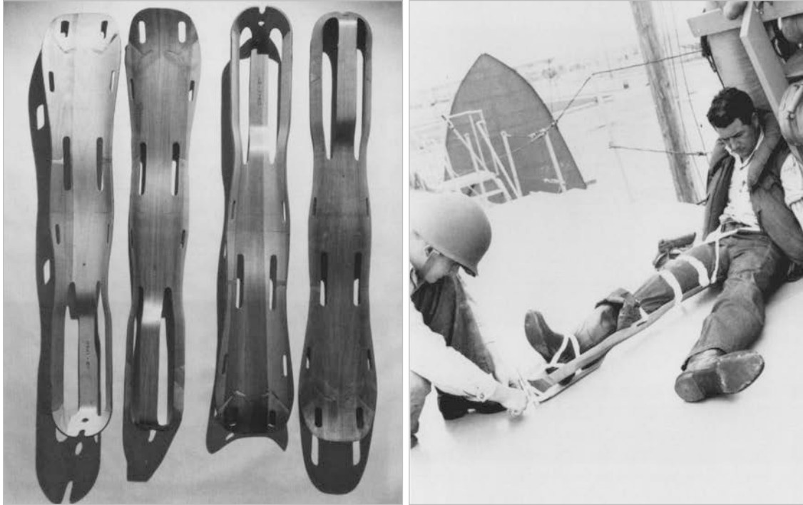
Left: The U.S. Navy placed its first order for the splints in 1942, and the Plyformed Wood Company (essentially functioning as the Eames Office) mass-produced the item as a subsidiary of the Evans Products Company. Right: A demonstration of the splint in use: Traction is applied to secure the broken bones and suspend the heel. (Demetrios -b Ch. 3 Pg. 112)
